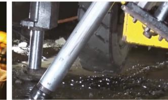
Sturdy stingers on front and rear to support drilling in steady position, that increases accuracy of drilling and decreases consumption of drill string.
