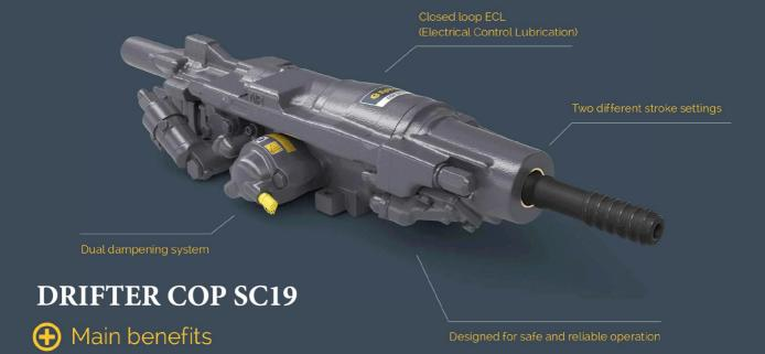
**Versatility** with two different stroke settings to optimize performance even as hole sizes and rock conditions vary
