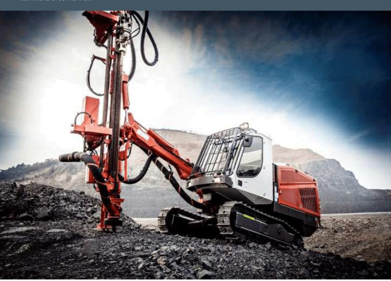
Tiger DG700 is a hydraulic, self-propelled, self-contained, crawler based surface drilling rig equipped with a cabin (F.O.P.S. and R.O.P.S.) and rod handling system.
